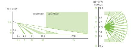
Diagram reflects sensor in first position. Adjust angle downward if mounting above 10 feet or to decrease gap directly under sensor.
